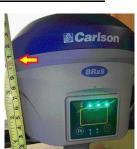
3) Then tap the Receiver tab and tap next to "Slant" and measure up to the line where the top Blue cap meets the bottom Grey housing as shown in the image to the right with the Arrow symbol to use for your Antenna height
